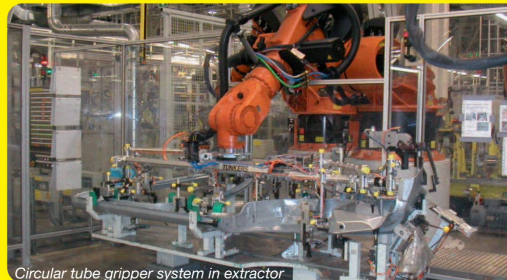
Circular tube gripper system in extractor
